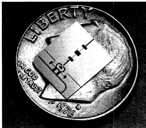
Fig. 6 Ka-band branchline mixer on a ferrite substrate
